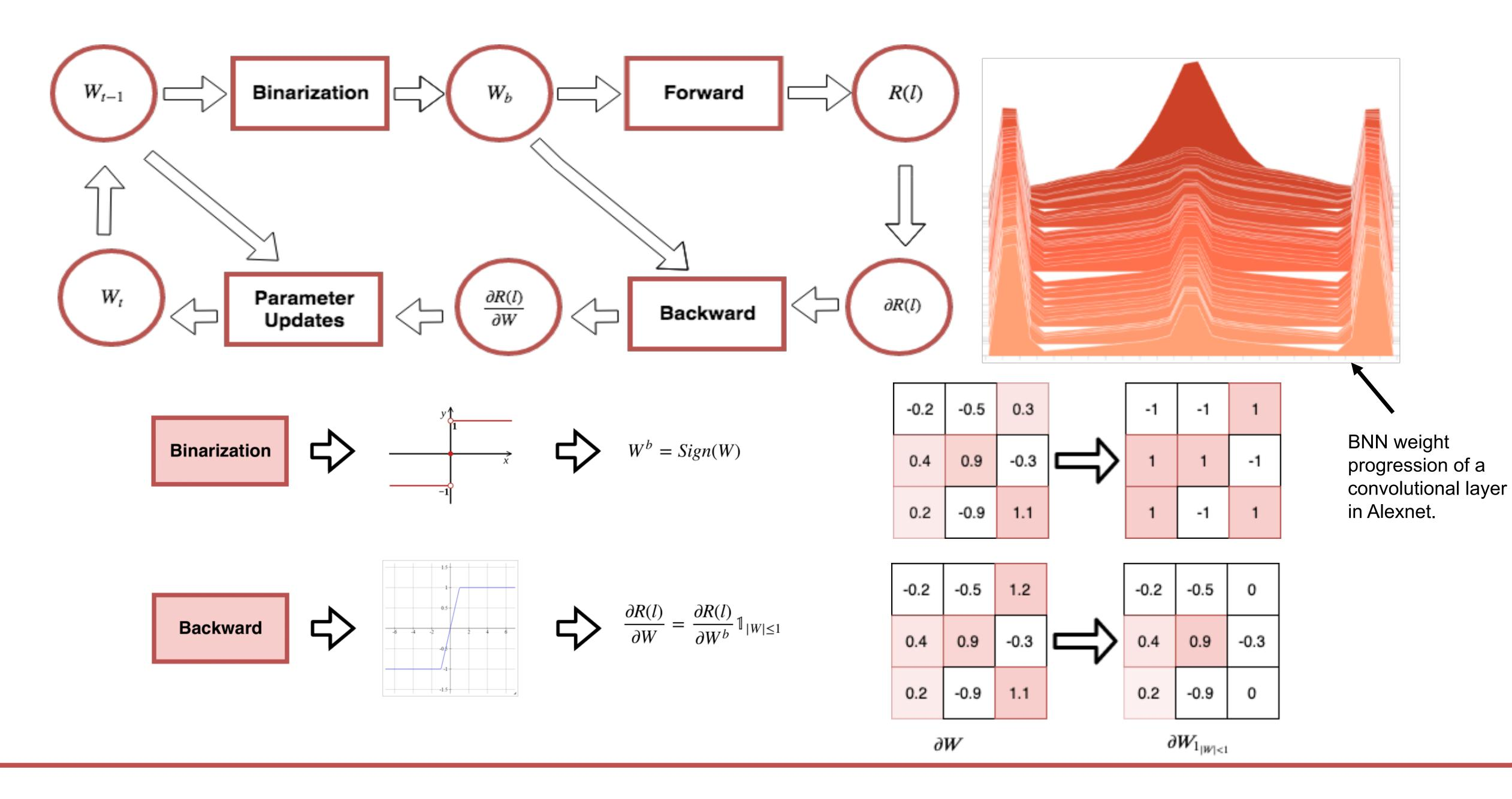
We present slight modifications to the BNN training method, by introducing trainable scaling factors, along with regularization terms to help train them through out the network. Additionally, a modified backward straight through estimator SwishSign is used.
